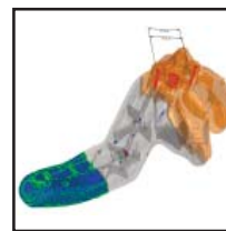
3D metrology and pore analysis of an automotive control arm
